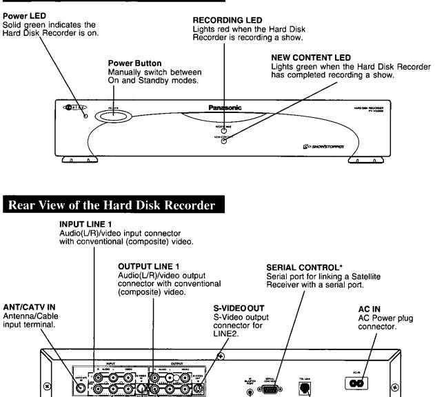
S-VIDEO INIR BLASTER PORT\*S-Video inputInfrared (IR) jack forconnector forcontrolling a DBS orLINE2.cable box with IR control.
