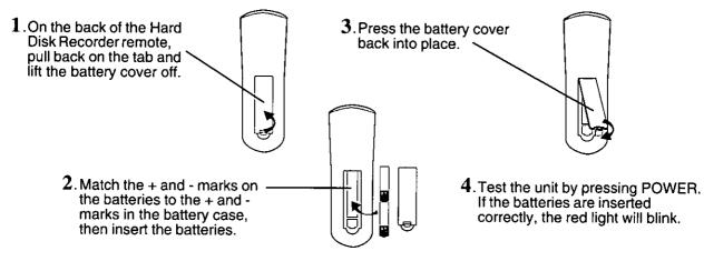
NOTE: Removing the batteries will not require you to re-program your remote control.
